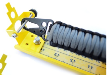
Threaded rod and nut can be used for various hooks, snaps, and accessories.
